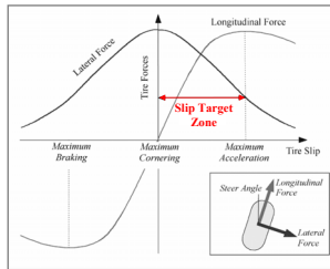
Typical behavior of lateral and longitudinal tire forces.
