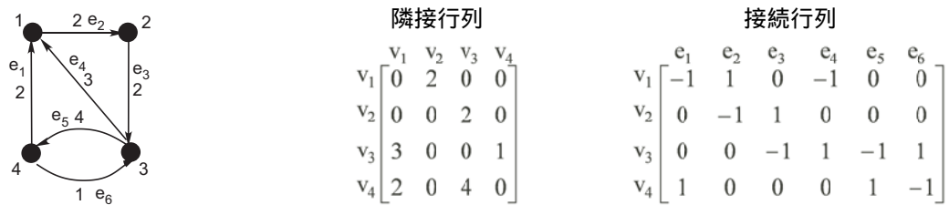
Fig. 7: adjacent matrix and incident matrix of weighted graph
